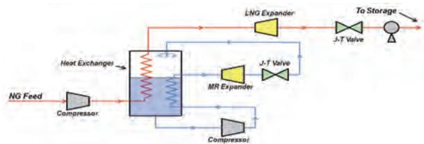
**Figure 3.** Liquefaction process with single phase cryogenic expanders.
