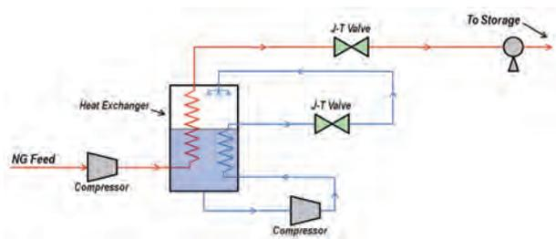
**Figure 1.** Simplified isenthalpic liquefaction process.
