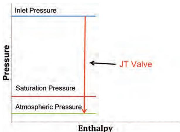
**Figure 2.** P-h diagram of J-T valve pressure reduction.
