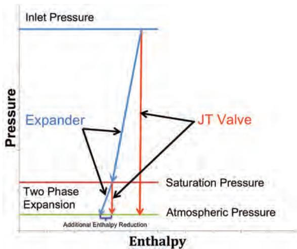
**Figure 5.** P-h diagram of two phase expansion.
