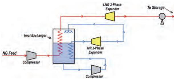
**Figure 6.** Simplified liquefaction process using two phase expanders.
