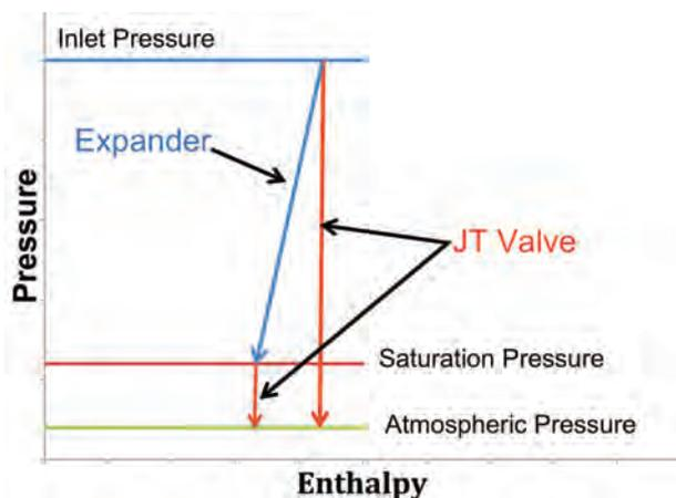
**Figure 4.** P-h diagram of liquefaction process with cryogenic expander.
