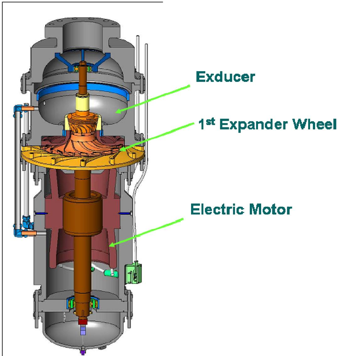
**Figure 3 - Ebara Two-Phase Expander Cross Section**
