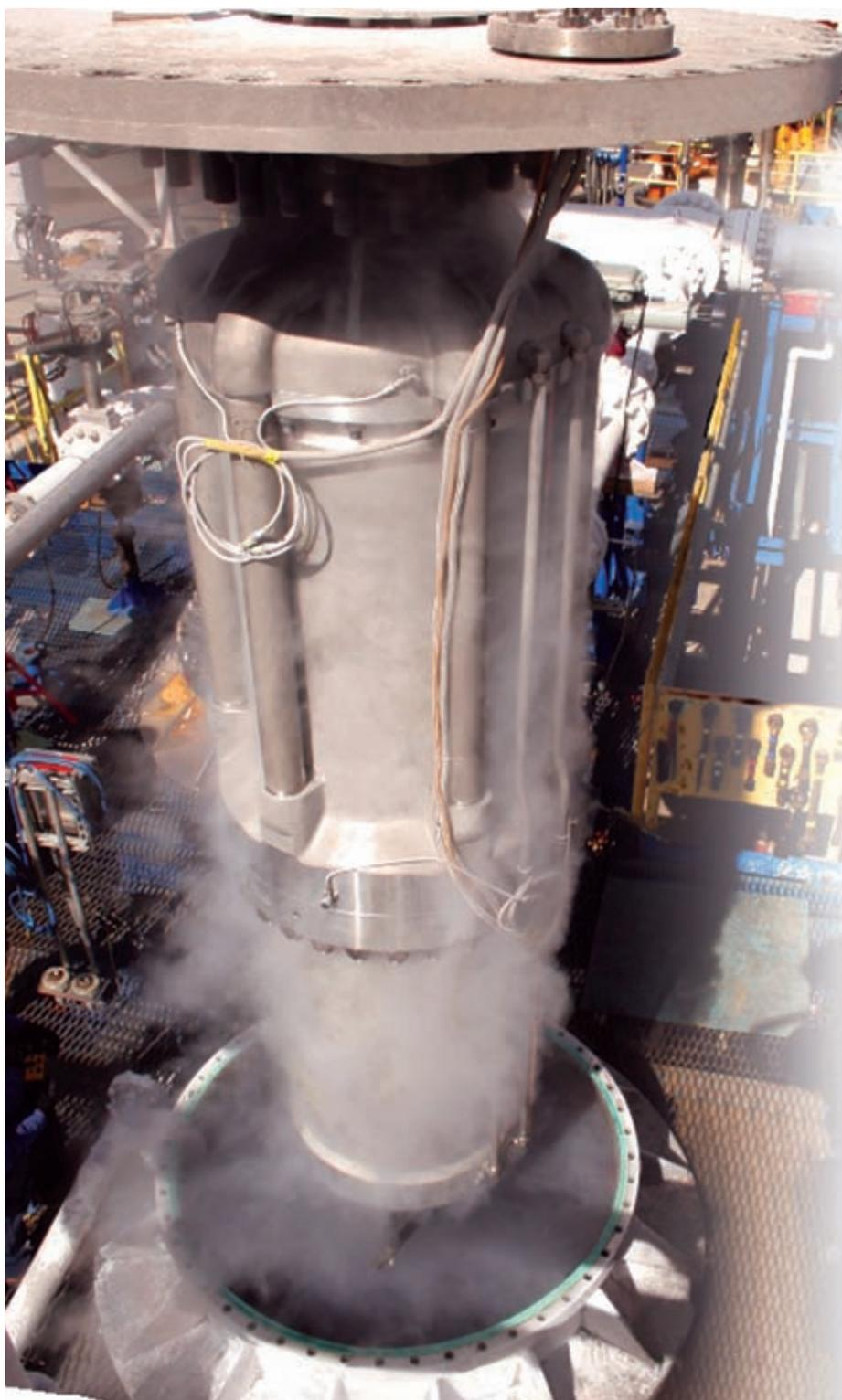
The large high-pressure pump can be used for send-out or vaporizer feed
