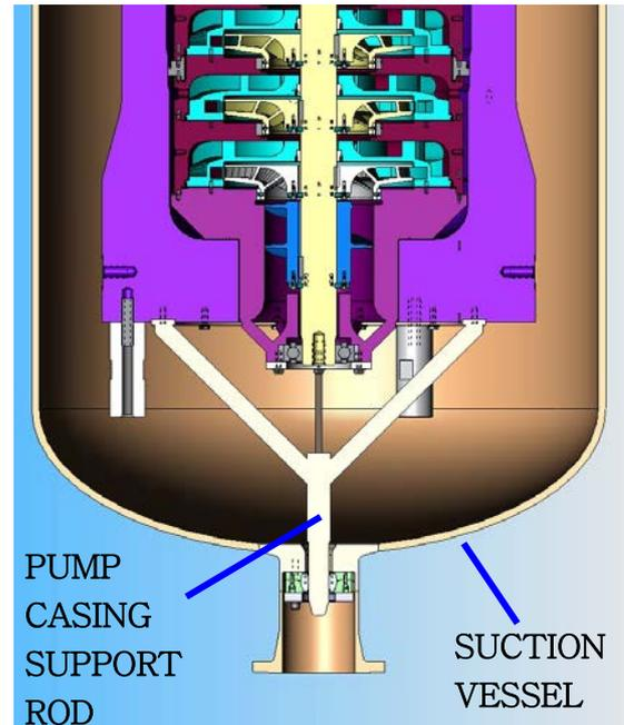
Figure 4 Pump casing support shown with the suction vessel.
