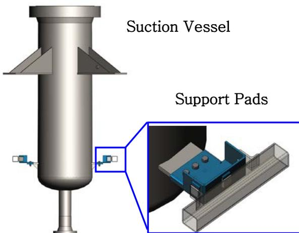
Figure 3 – Vessel Mounted High Pressure pump with lower support pads.
