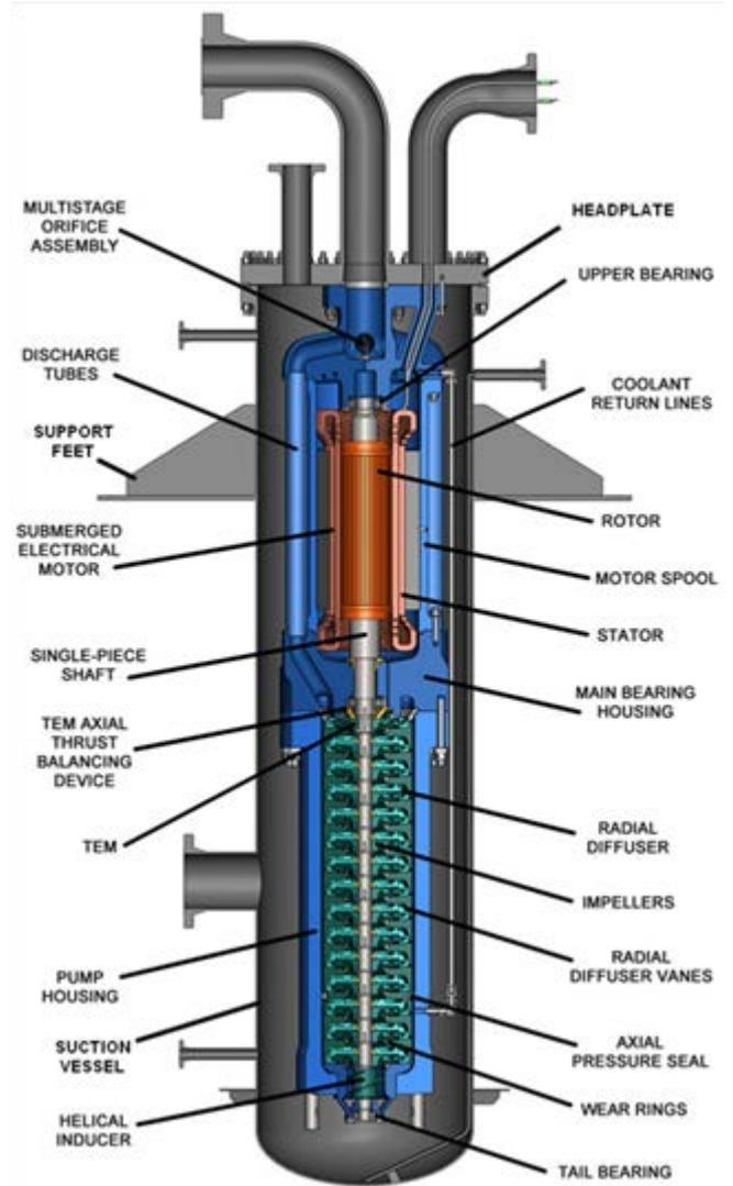
Figure-2 Cross Sectional View of Typical Suction Vessel Mounted High Pressure Pump.
