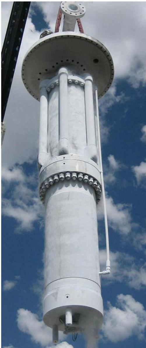
Figure-1 Typical Vessel Mounted High Pressure Pump during removal from the vessel.
