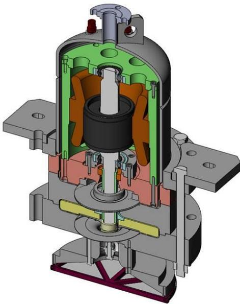
Figure 3: Small Scale Marine Pump
