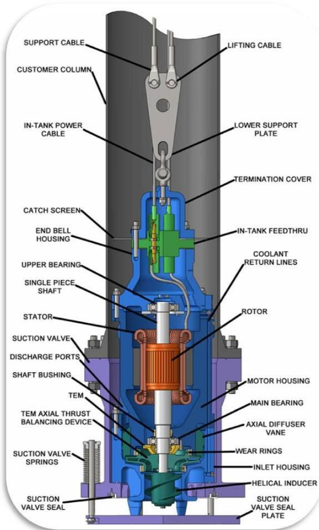
Figure 1: Typical In-Tank Retractable Type LNG Pump
