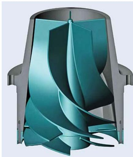
**FIG. 15** Two-phase draft tube.
