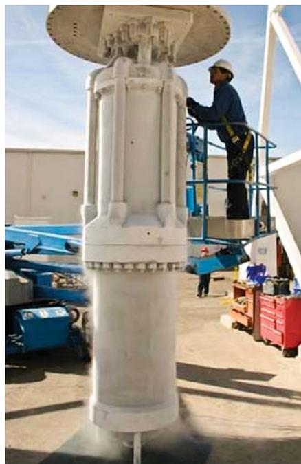
**FIG. 1** Nine-stage submersible LNG sendout pump, post-performance test.
