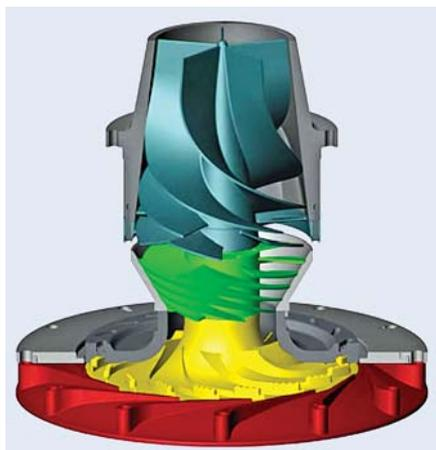
**FIG. 11** Two-phase hydraulic assembly.
