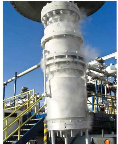
**FIG. 16** Two-phase expander post performance test.
