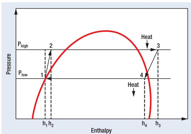
**FIG. 4** Four steps of an ideal Rankine cycle.
