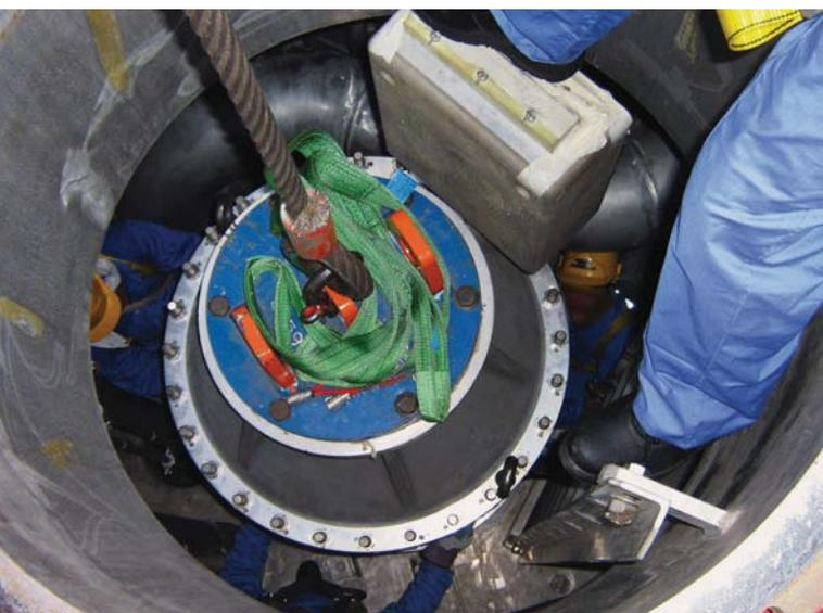
*Lifting an Ebara cargo pump clear of an LNG carrier tank for servicing*
