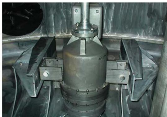
*In addition to two cargo pumps each LNG carrier tank is provided with a spray pump*
