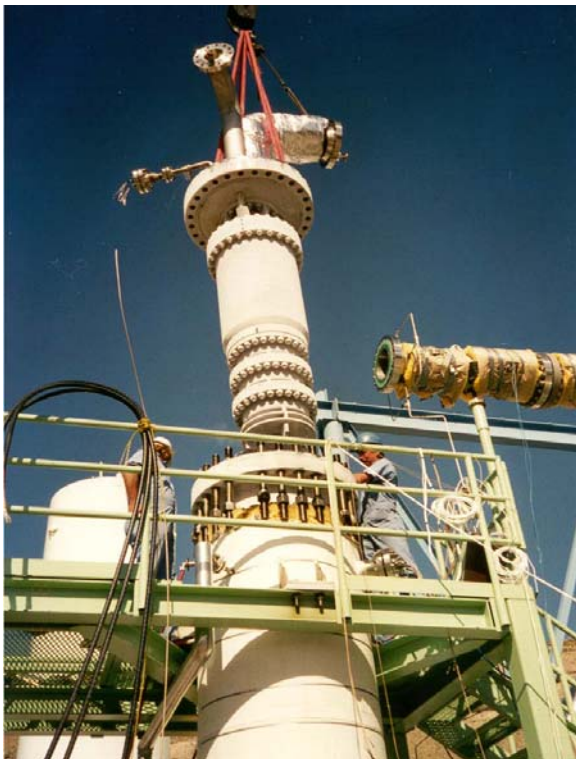
Figure 7: Variable Speed LNG Expander on the Test Stand
