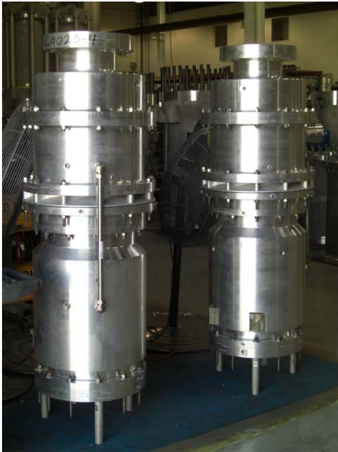
Figure 19: Two-Phase Expanders at the Manufacturing Plant
