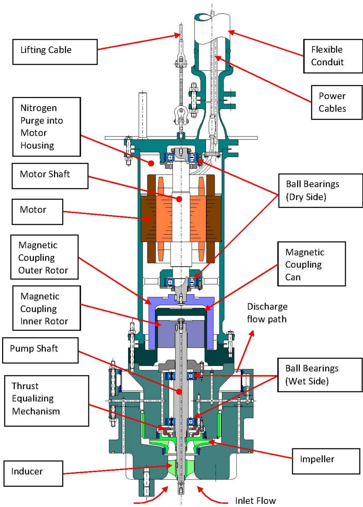
Figure 2: Pump Design with Magnetic Coupling
