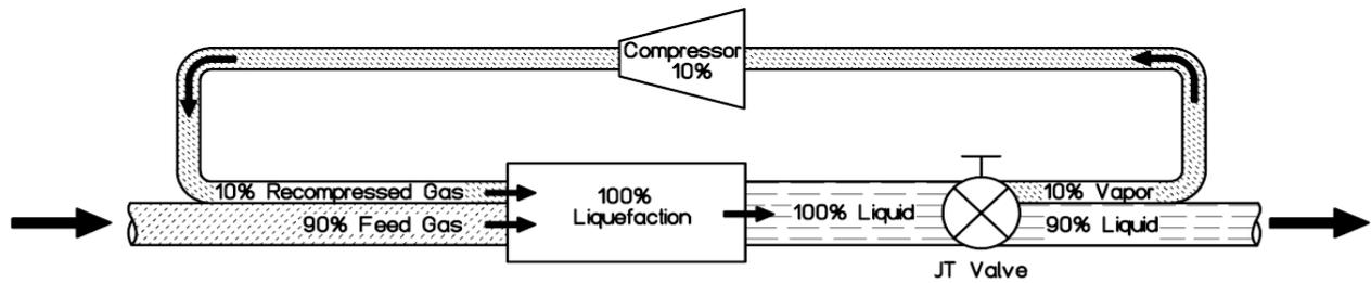
**Figure 4a: Liquefaction Process using a Joule-Thomson Valve**
