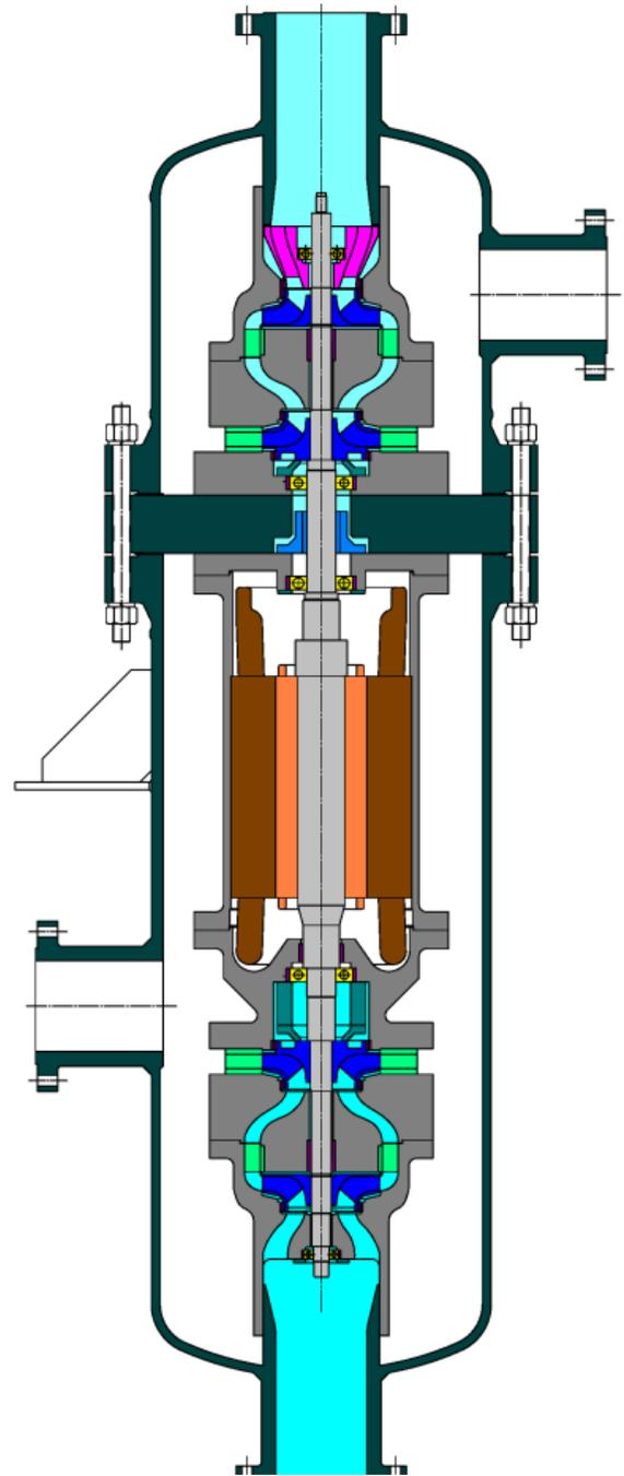
Fig. 3: Compact Expander-Expander Configuration
