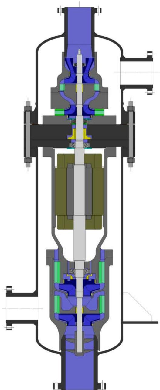
**Fig. 1: Compact Pump-Expander Configuration with Submerged Motor/Generator**
