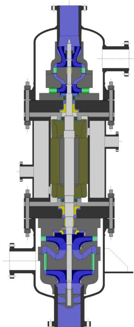
**Fig. 2: Compact Pump-Expander Configuration with Separated Motor/Generator**
