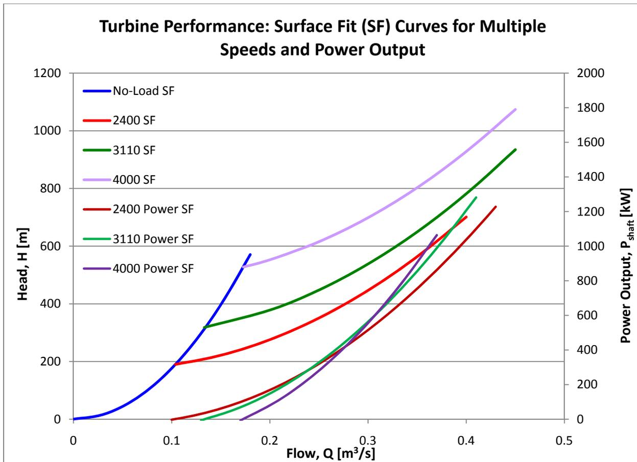
**Fig. 3: Shaft Power Surface Fit Curves with Turbine Performance**
