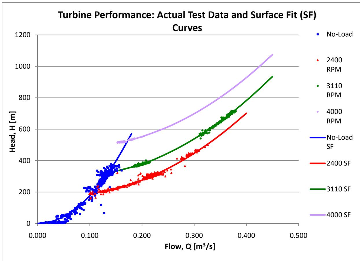
Fig. 2: Actual Test Data and Surface Fit Curves
