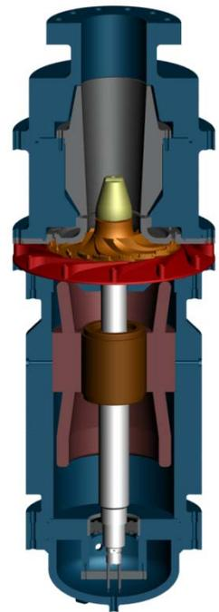
**Fig. 1: Turbine Solid Model**
